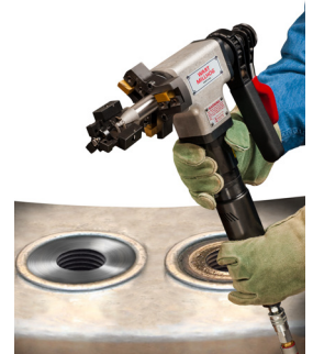
Bolt hole resurfacing is prepared using a standard Wart MILLHOG and cutter blades.
