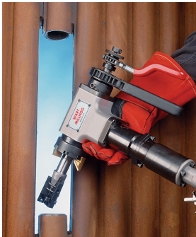
The Wart needs a minimum of 2.625" to fit between tubes in a boiler tube waterwall.
