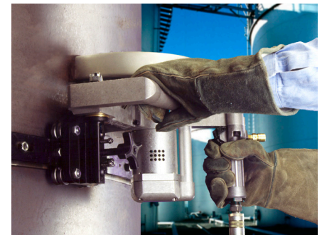
The Flex Track attaches to straight, contoured, cylindrical and serpentine surfaces for making accurate square cuts with no "HAZ".
